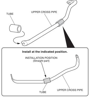
8. Loosely install the upper cross pipe as shown.
