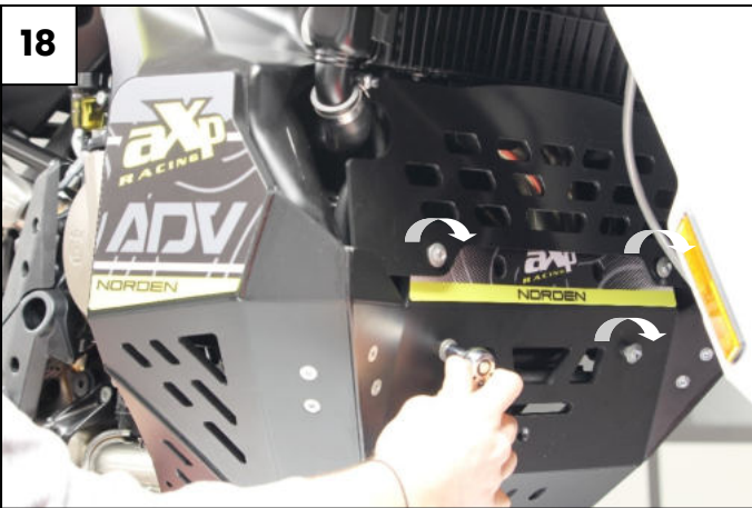
Tight all four front screws (18) Tight the rear fixation points on left (19) and right side (20)
