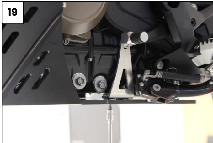
Tight all four front screws (18) Tight the rear fixation points on left (19) and right side (20)
