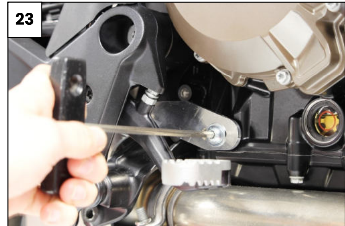
Tight all the others screws : The 8x16mm on left side (21) the 8x50mm and the 8x16mm on the right side (22-23) and it's done !
