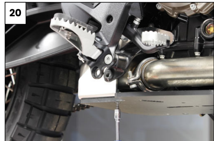
Tight all four front screws (18) Tight the rear fixation points on left (19) and right side (20)
