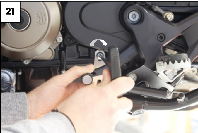
Tight all the others screws : The 8x16mm on left side (21) the 8x50mm and the 8x16mm on the right side (22-23) and it's done !
