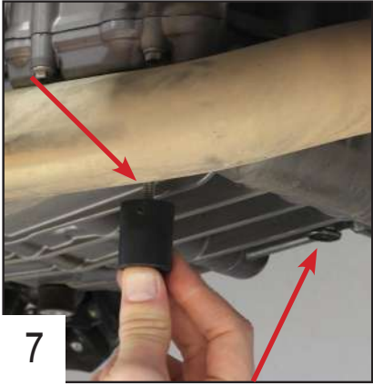
7 Screw the two silent blocks in the engine.
