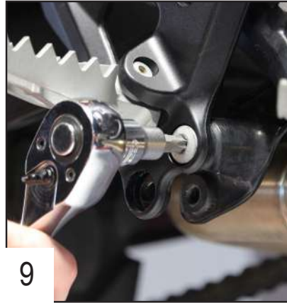
9 Untight the OEM screw, without removing it completely.
