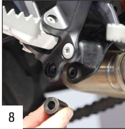
8 Remove the OEM spacer under the footpeg.
