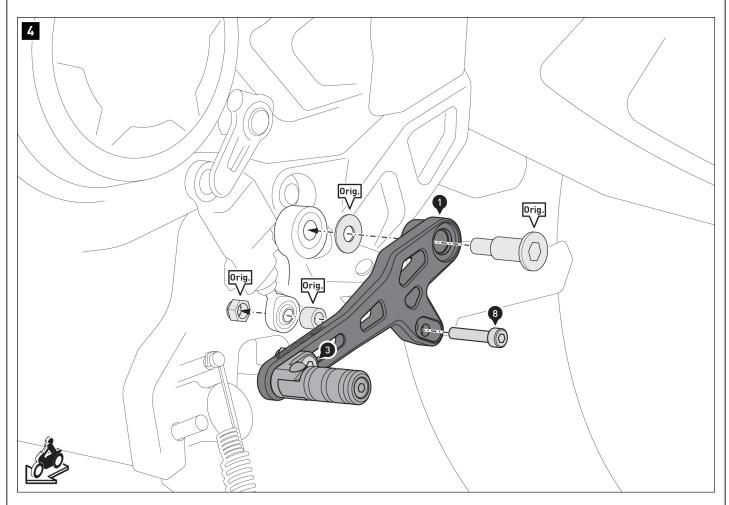
Screw the gear lever (1) to the original parts (Orig.) on the vehicle and the shift rod.
