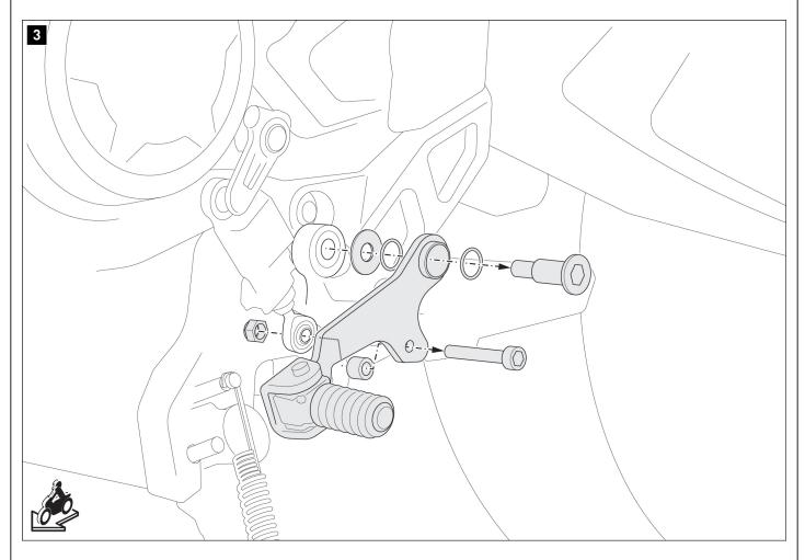
Loosen the nuts and bolts and remove the original gear lever from the vehicle.
