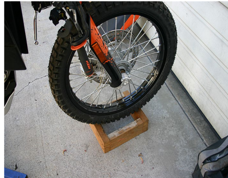
Blocking both front and rear wheels is a good idea to prevent "roll-aways" once the triple clamp is removed
