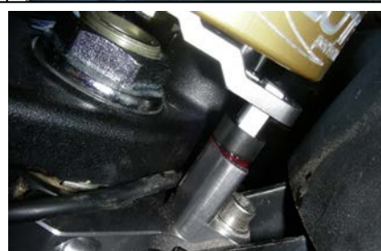
Tower pin greased & installed correctly
