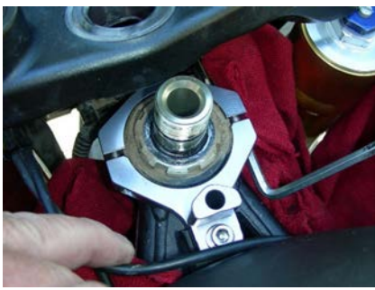
Tighten the bolts so the gap remains equal on both sides and the tank bolt should not be tight yet.
