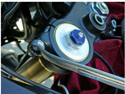
Don't forget to tighten the fork pinch bolts after triple clamp goes back on.
