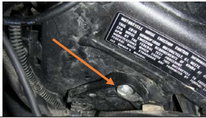
Remove the cable mount on the left side, below this label, to give the cables room to remove triple clamp
