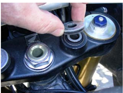
Retain stock rubber/washer between the Sub assembly and triple clamp
