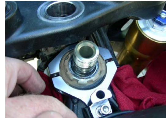
Lift the triple clamp up just high enough to install the new frame bracket.
