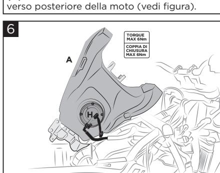
**Connect the connectors to the pump (H) first to mount the tank (A). ATTENTION: when tightening maximum torque spec 6Nm.**
