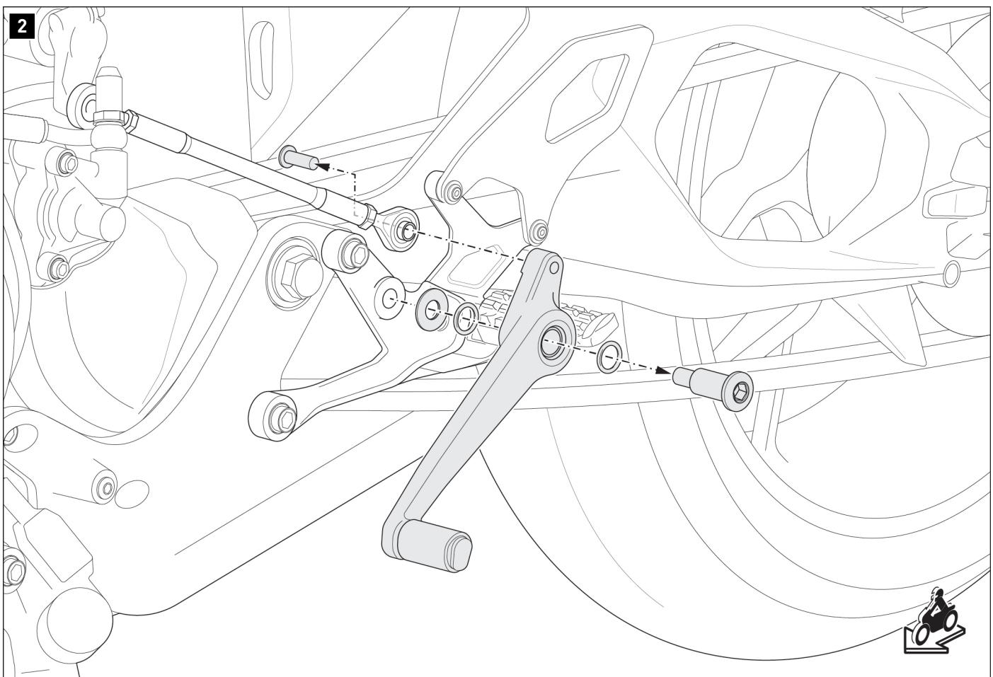
Loosen the parts indicated; remove the original gear lever from the vehicle.
