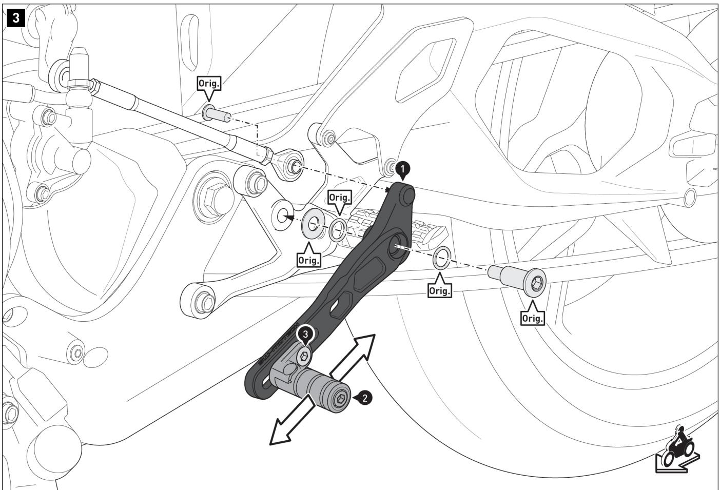
Screw the deflection rod to the gear lever (1).
