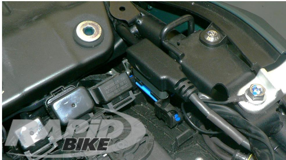
The connectors joined in this way are not waterproof. Using insulating, waterproof and temperature-resistant tape (not supplied in the kit), proceed to tape the connectors at their junction so as to prevent the entry of water and humidity.
